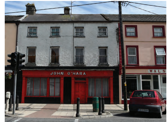
Plate 16: John O'Hara: This is a significant building due to the extent of surviving historic fabric of quality – the fine timber shopfront, the upper floor wet dash and whitewashed plaster; the historic windows. Note also the elegant shopfront of Walsh's to the right.
